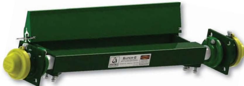
The Super-G's unique "pass-through" mainframe design allows material to freely fall through it, keeping your systems online with little to no maintenance. This system is based on the same heavy-duty mainframe and Perma-Torque tensioner as our Eraser system. Choose either a urethane or tungsten carbide blade.
