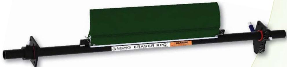
The Eraser RPQ system uses the same simple and effective spring tensioning unit as the Eraser PQ, with a 7" tall polyurethane blade, giving you more wear life and allowing for installation on systems with a larger diameter head pulley.
