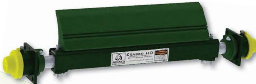
The Eraser HD is designed to withstand heavy vibration. This system has a reinforced mainframe and a heavy-duty channel attachment design. It utilizes a series of 6" wide x 7" tall polyurethane blade segments that conform to crowned head pulleys.
