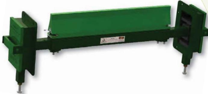
The XTC is one powerful reversing conveyor cleaner. Choose from polyurethane, tool steel, stainless steel or tungsten carbide blades. The system can handle wet, dry, sticky or slimy conditions. The unique Web-Torque tensioner has enough give for mechanical splices and the flow-over blade design reduces material build up.
