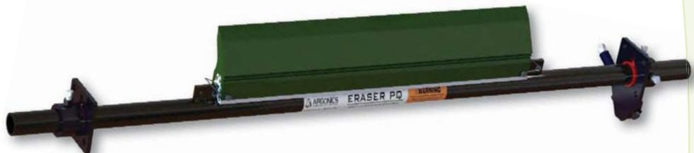
The Eraser PQ (Pit and Quarry) system is an economical cleaner designed for performance and reliability. With a simple and effective spring tensioning unit, it uses our 6" tall polyurethane blade and requires little to no maintenance.
