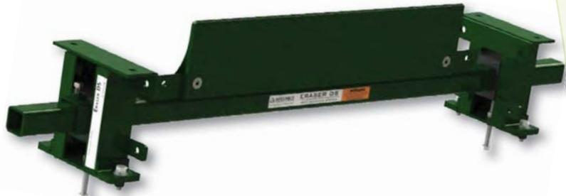
The Eraser DS is an economical version of our XTC cleaner, with a .19" thick, 2"x 2" powder-coated tube stock steel mainframe for strength and durability. The DS uses the same polyurethane and tungsten carbide blades as the XTC. The tungsten system is urethane-free for use with high-temperature materials.
