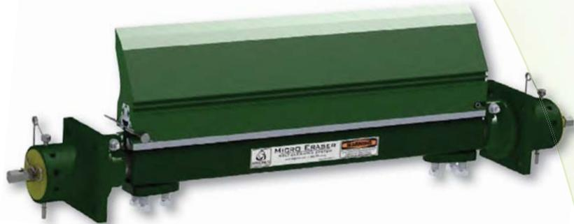
The Micro Eraser is your answer for portable equipment with tight clearance issues. Designed with our 6" tall polyurethane blade, it works best on belts up to 48" wide with head pulleys of 28" diameter or less. This economical but powerful system uses our patented Perma-Torque™ tensioner.
